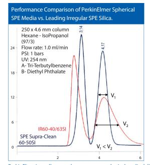
PerkinElmer's smaller, more homogeneous, spherical media deliver sharper, narrower peaks for faster, more accurate sæmplysis
