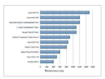
Compared to other industry leading SPE materials, our Extreme Capacity (XC) and Extra Wide Particles (XWP) lead market in surface area. This allows for higher capacities at lower bed weights.
