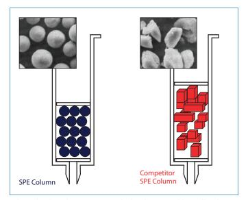
Spherical media and consistent particle distribution enable smaller elution volumes and better, more reproducible action, purification, concentration and recovery.
